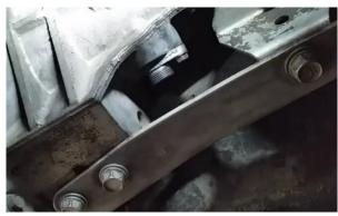
5. Find the bolts at the rear of the PPF holding the PPF to the differential housing. Loosen the bolts most of the way, then tap with a hammer to dislodge the captured nuts.
